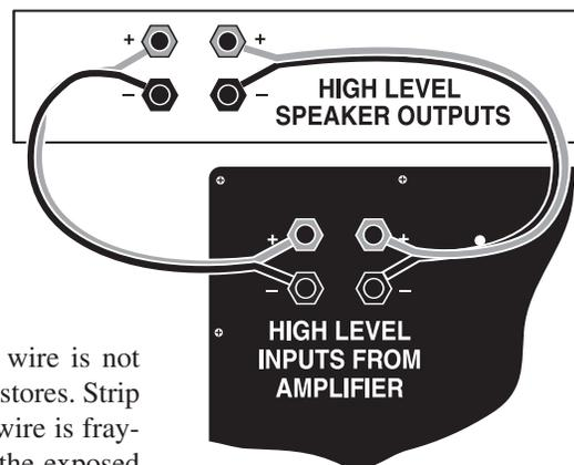
Run the wires from your system's amplifier to the subwoofer's HIGH LEVEL INPUTS. For each channel, run wire from the red (+) outputs on the amplifier to the subwoofer's red (+) inputs, and from the black (-) outputs on the amplifier to the subwoofer's black (-) inputs. Make sure the black amplifier outputs are "true ground." Bridged outputs cannot be used.
