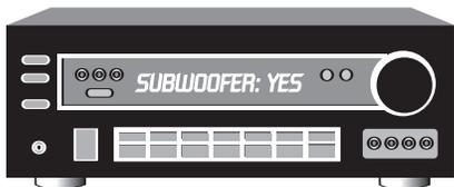
Set your controller to enable subwoofer output. To do this, go to the SPEAKER SET-UP or BASS MANAGEMENT menu and set the SUBWOOFER to ON or YES. All the speakers should be set to SMALL if possible. This directs the deep bass from the satellites to the subwoofer, freeing them and their amplifiers from the rigorous demands of reproducing bass.
